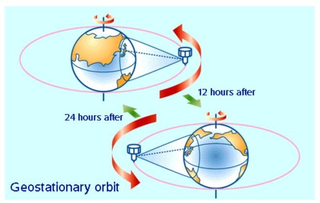
A satellite that appears to remain in the same position above the Earth is called a "geostationary satellite."
