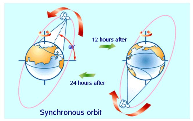
A satellite in a synchronous orbit goes around the Earth once a day returning to its original position
